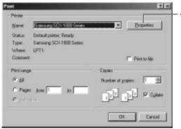
To take full advantage of the printer features, click the Properties button. For more information about Properties, see 'Using Features in the Printer Driver' on page 5-7.
